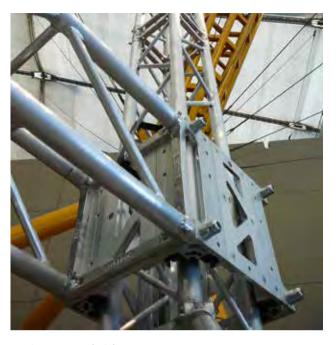
Base module for towers with frame of 29 cm sided square truss. The system comes furnished with detachable foldaway stabilizers. The multistandard sleeve block has 16 gliding wheels of high density rubber. Each foot moves both in pan and tilt so adapting to all terrain. The entire system, excluding the central truss, is formed of assembled parts, without any weldings.
