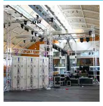
The Towerlift 3 hoist system occurs by manual winch with steel cables. The sleeve block functions as default component also for the Unitower and Varitower models. Each side can accommodate either square truss of 29 cm or 40 cm sides, or triangular truss of 29 cm sides. A triangular truss of 40 cm may also be connected by substituting the appropriate central support plate.
