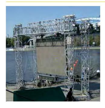
Free-standing mid-range LED support frame incorporating Varitower 3-40 and QL52A horizontal beams for screens up to 2,000 kg.
