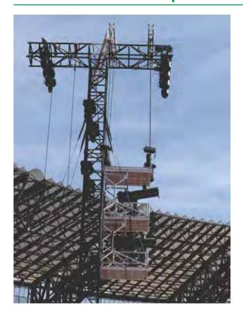
LITEC offers a new system for followperson during the show. The system provides a platform with a 200x150 cm space to allow the operator to follow the artist during the show. The structure incorporates the concept of LIBERA that reduces transport volume to the maximum.
