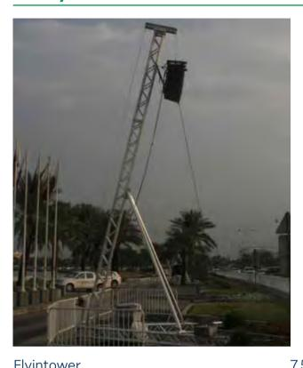
Support Tower for audio systems consisting of a QX30SA structure, suitable for lifting loads of up to 600 kg to a height of 9.5 metres.
