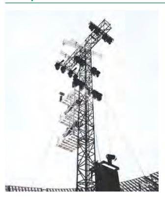
Support tower for audio systems or follow spot system. Designed in QL85A, this new Flyintower is suitable for 8,000 kg loads and can reach the height of 15,5 meters, thus ensuring sturdiness and rigidity on relevant heights. It also utilized the ballast system to stabilize itself and it creates a free area on the front to simplify the system for loading.
