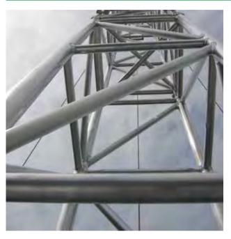
Support tower for for audio systems. Designed in RL105A, this new Flyintower is suitable for 2,000 kg loads and can reach the height of 16 meters, thus ensuring sturdiness and rigidity on relevant heights. It also utilized QH30SA trusses as stabilizing elements and is equipped with fork connections.
