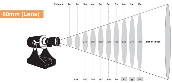
Ratio for Distance 1,4:1 (Image Size - 60mm Lens) no other light sources nearby The Object Diameter is 42mm
