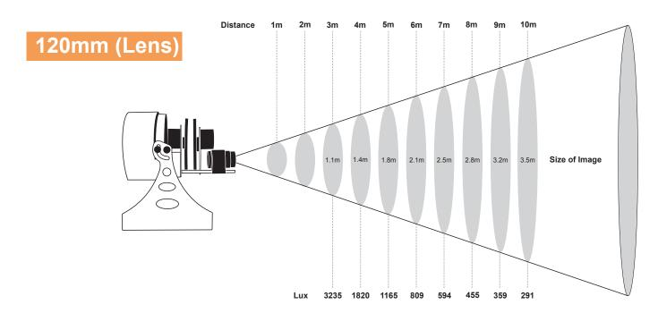
Ratio for Distance 2,9:1 (Image Size - 120mm Lens) The Object Diameter is 42mm
