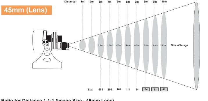
Ratio for Distance 1,1:1 (Image Size - 45mm Lens) The Object Diameter is 42mm
