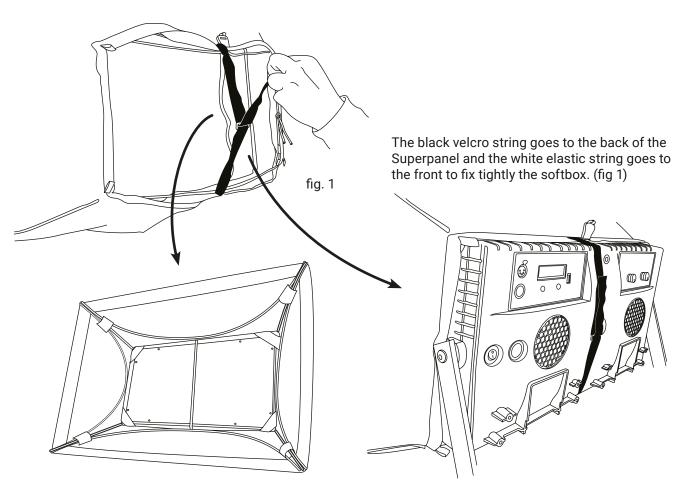
Tighten the elastic to close the gap between the softbox and the Dayled PRO until it's fixed (fig. 2).
