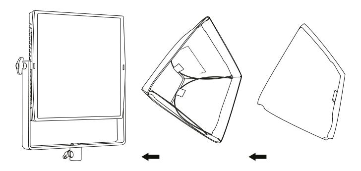
To secure the softbox at the Superpanel 30 pass the velcro string at the edges of the panel and make sure to thighten it. (fig 1)
