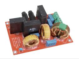
[ \* all fixtures of this series ] High immunity to voltage overloads thanks to the use of a 10KV-10KA Surge Protection Module capable of withstanding voltage and current pulses up to 10.000Volt and 10.000Ampere.
