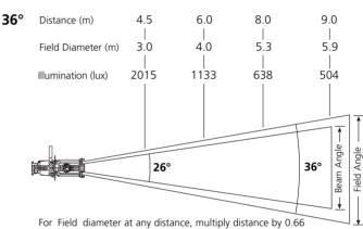
For Beam diameter at any distance, multiply distance by 0.00
