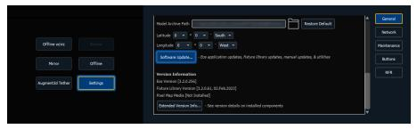
3. Insert the USB storage device and scroll down until you can press **(Software Update...)**. Any valid Eos installers detected will appear in a pop-up list.
