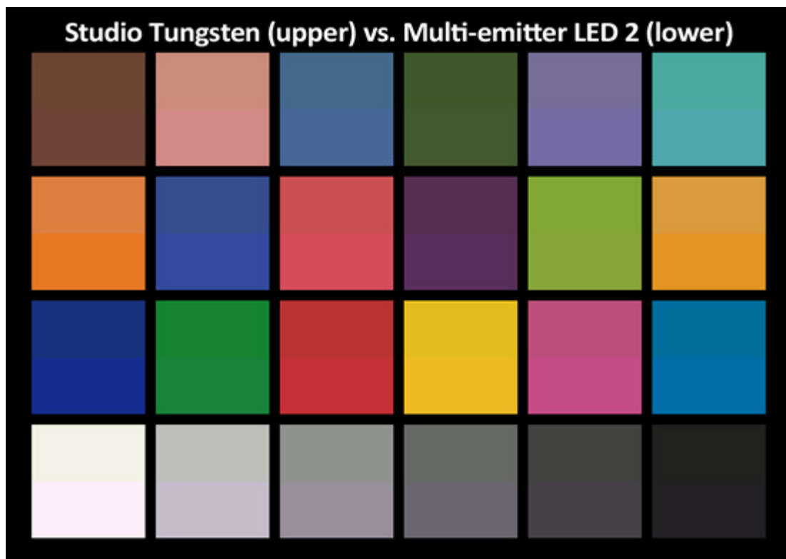
Split Macbeth chart: each color patch shows the visible effects of studio tungsten light in the top half of the patch, and a representative multi-emitter LED lighting instrument in the bottom half.
